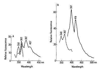
Figure 2. Fluorescence excitation (---) and emission (-) spectra of (A) 4,5- and (B) 7,8-dihydrodiols of BaP isolated from algal medium extract. Only the long wavelengths of the excitation spectra are reported.
