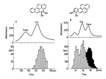
Figure 1. HPLC chromatographs of standard *cis*- and *trans*-dihydodiols cochromatographed with (A) 4,5- and (B) 7,8-dihydrodiols isolated from algal cultures incubated with <sup>14</sup>C-BaP. Open bars represent radioactivity extracted from algal medium. Closed bars represent addition of synthetic <sup>14</sup>C-*trans*-7,8-dihydrodiol BaP spike (1500 dpm) to the medium extract.
